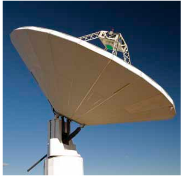
A dedicated 12-metre antenna has been built at CSIRO's Parkes Observatory and it is now being used to test ASKAP technologies including novel receivers (phased array feeds). Credit: David McClenaghan, CSIRO.
