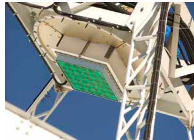
ASKAP's prototype phased array feed on the Parkes Testbed Facility. Credit: David McClenaghan, CSIRO.
